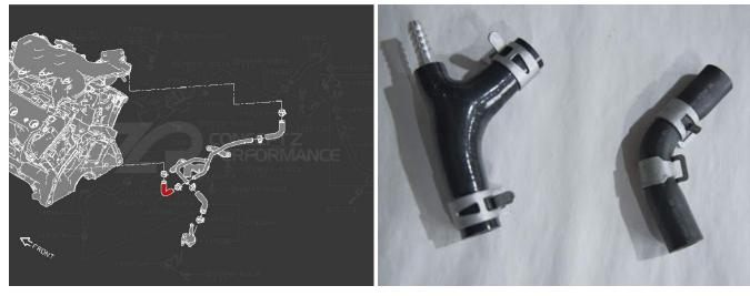
15. Install the CZP silicone Y-shaped replacement hose using the supplied 16mm spring clamps.
