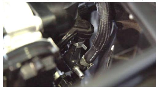
16. Connect one side of the 6mm silicone vacuum line and run it up to the center of the engine and connect it to the 6mm side of the 6mm to 2x 3.5mm plastic T fitting, making sure to secure both ends with a ziptie.
