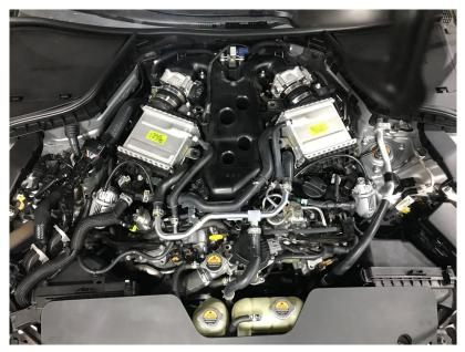
14. Using pliers, remove the two spring clamps holding the short angled vacuum hose that goes downward from the rear drivers side of the plenum to a hardline mounted to the back side of the engine. Be careful as the fitting on the plenum is only plastic.
