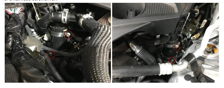
5. Disconnect the Intercooler MAP sensors on both sides near the throttle bodies
