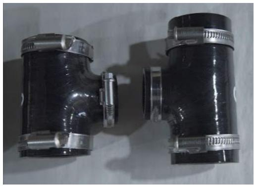
8. Install the BOV couplers so that the open port on the coupler faces towards the headlight on the side it is mounted (drivers side points to the drivers side headlight and passenger side faces the passenger side headlight) but don't tighten the two clamps yet as slight adjustments for correct fitment may be necessary.
